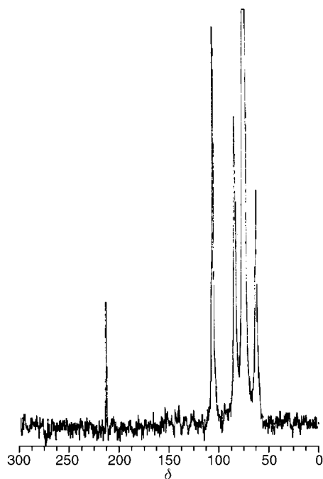
Fig. 1 Solid state ^{13}\text{C} CP/MAS NMR spectrum recorded at 64.7 MHz for a ^{13}\text{C} enriched sample of the \text{Cr}(\text{CO})_6/\gamma\text{-CD} adduct with cross polarization (contact time 5 ms) and a recycle delay of 3 s. The sample spinning speed was 5000 Hz.
